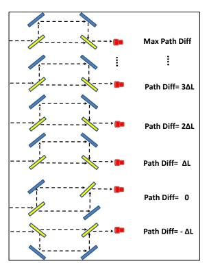
Figure 6: Array of Mach Zehnder interferometers with path difference fixed at different values.
