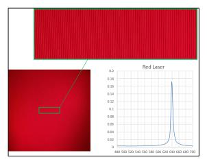
Figure 8: FrinGOe image of fringes of red laser and its processed FTIR spectrum
