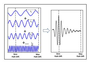
Figure 4: Resultant interferogram for light with broadband spectrum
