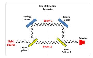
Figure 5: Mach Zehnder interferometer
