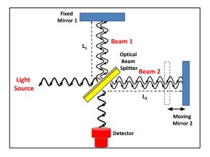
Figure 1: Scanning FTIR interferometer
