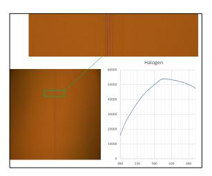
Figure 9: FrinGOe image of fringes for halogen light and its processed FTIR spectrum
