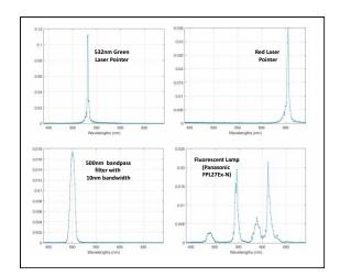
Figure 10: Examples of measured spectra using 400fringe FrinGOe on iPhone 5s camera
