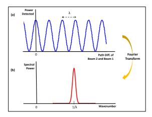
Figure 2: Sinusoidal interferogram for a monochromatic light of wavelength  $\lambda$  and its corresponding spectrum in wavenumber
