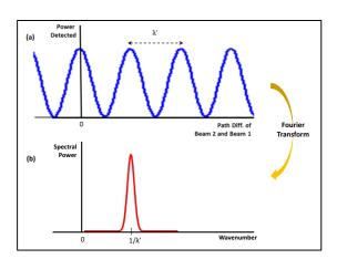
Figure 3: Sinusoidal interferogram when wavelength change to  $\lambda'$  and its corresponding spectrum in wavenumber
